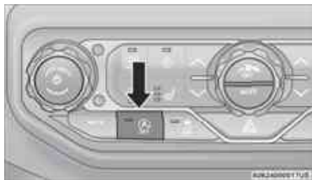
Stop/Start OFF Switch
